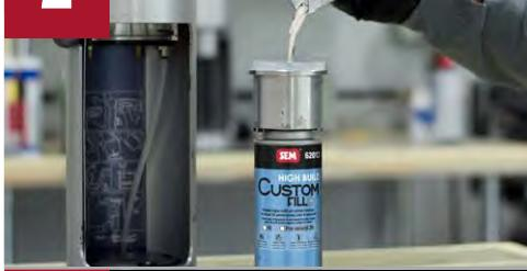
Remove the tip from the aerosol. Press the cylinder/cap assembly on top of aerosol blank. Fill the clear plastic cap with paint to the fill line.
