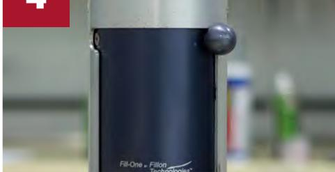
**FOR MANUAL MACHINE:** Rotate crank until it stops and then rotate in the opposite direction until it stops. **FOR PNEUMATIC MACHINE:** After closing the door, the machine will fill the aerosol. Wait until the machine is silent. Open the door and loosen pedestal to remove assembly from the machine.
