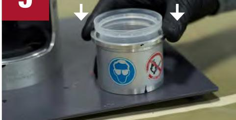
Remove cylinder/cap assembly from machine. Twist gently to remove cylinder from can. Hold cylinder and press down on a hard surface to remove cap. Replace tip.
