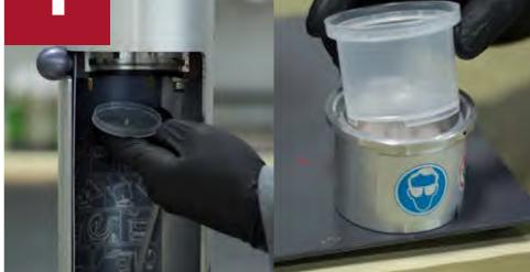
Remove disc from cap and insert over piston inside the fill machine. Place clear plastic cap into the **Fill Cylinder**. Press down and rotate cap until it drops into place.
