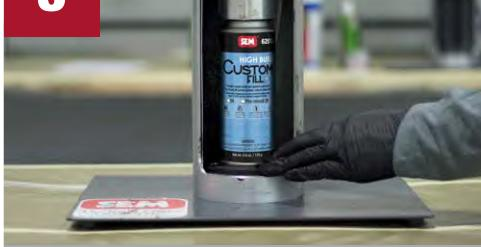
Place assembly into machine. Hold cylinder and cap assembly in place and tighten pedestal on bottom. Close door on **Custom Fill Machine**.
